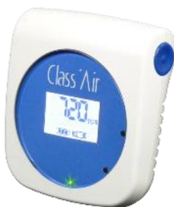
Figure 69 – Class'air sensors indicating the air stuffiness from coloured leds
