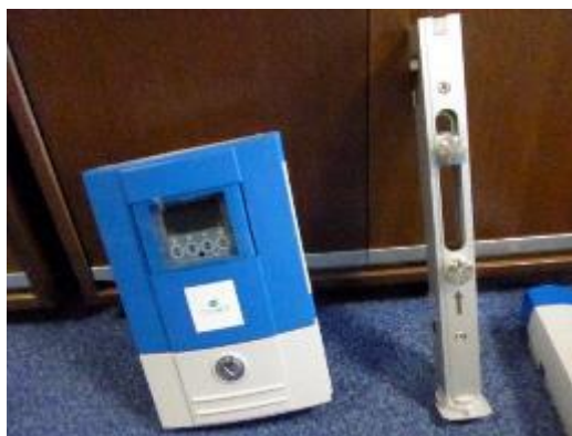
Figure 99 – Ultrasonic flowmeter used to monitor the water consumption in the toilets before and after replacing the health facilities
