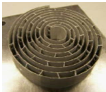
Figure 2-12. Industrial part manufactured by SLM technology by IK4-LORTEK research centre.
