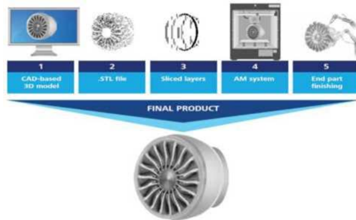
Figure 3-1. AM Process flow. [39]
